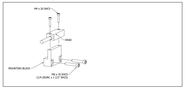
2.4 The gap between the reader head and the scale should be 0.5mm ± 0.1mm this is set with the shim provided, align reader head as shown.
